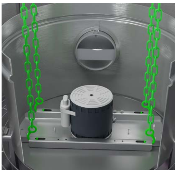
Model VCU (Motor support plate features four lifting points)
