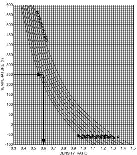
**Example 4:** Select a fan to deliver 8500 CFM at  $2^{1}/_{2^{"}}$ SP at 5,500 ft elevation at 250°F. From Table 1 the factor for 250°F is 1.34 and from Table 2 the factor for 5,500 ft elevation is 1.22. The overall factor is obtained by multiplying these factors: 1.34 x 1.22 = 1.63. To use a fan manufacturer's performance tables, convert the SP to standard air:
