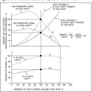
This density ratio must always be considered when selecting a fan from a manufacturer's catalogs or curves.
