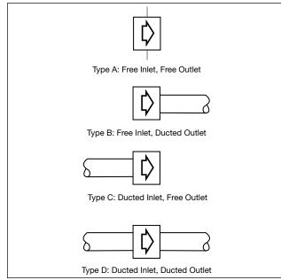
Products that are rated and certified by AMCA must illustrate that they have been rated by one of the installation types shown above.
