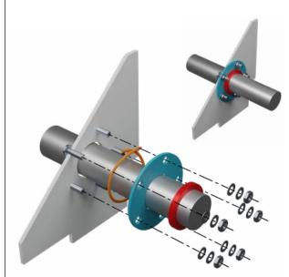
**Theory of Operation** — The axial type seal is compressed against the Teflon® wear plate. It seals when compressed to a specific amount. The friction fit of the V-ring seals the shaft.
