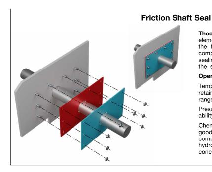
Theory of Operation — The friction shaft seal element is provided with a diameter smaller than the fan shaft. When the shaft seal outer plate compresses it against the fan housing, the
