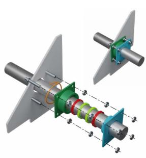
Theory of Operation — The stuffing box is sealed to the fan housing with PTFE joint sealant for a gasketing material. The packing materials are two flexible graphite split rings sandwiched between two carbon yarn anti-extrusion rings. The outside hex nuts force the outside packing plate into the stuffing box, expanding the graphite rings to provide a leak tight seal.
