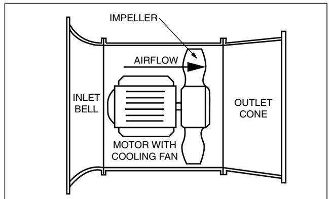
with corrosive chemicals or explosive vapors. They can be mounted in parallel for higher airflows or they can be staged in series to increase their pressure capabilities. Also, as mentioned under the panel fans, using larger hub-to-tip ratio impellers increases the tubeaxial fan's ability to work against pressure for a given speed or conversely enables the fan to work against the same pressure at a lower speed.
