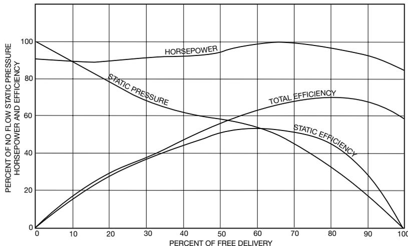
static pressure capability of the industrial panel fan over the commercial fan. Also note the higher efficiencies attained by this fan. Now compare the industrial panel fan performance (Figure 7) against a similar size tubeaxial fan (Figure 10). We can see that there is a negligible performance difference between a well designed industrial panel fan and a tubeaxial fan.
