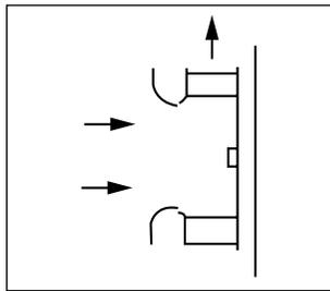
The axial flow fan increases the air velocity through rotational or tangential force, which produces velocity pressure (VP), kinetic energy, with a very small increase in static pressure (SP), potential energy.
