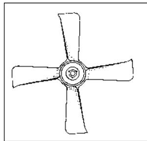
Figure 6. Medium Width Stamped Steel Impeller
