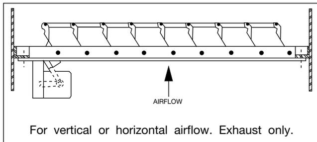
Another advantage of the motor operated damper is that when power is off the spring return ensures positive closing of the blades and is not influenced by stray eddies or air currents.
