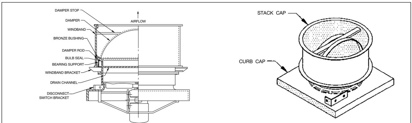
In addition to exhaust applications, square, rectangular and circular automatic backdraft dampers are also used in certain duct systems to function as check valves to prevent reverse airflow through a fan during shut down. This is of particular importance in parallel fan systems, where the fans are cycled independently, to prevent “windmilling” of the fan that is not in operation.
