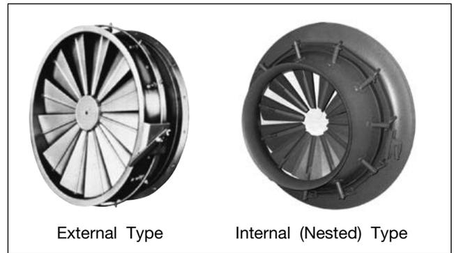
both a resistance and flow modifying effect by pre-spinning the air before it enters the fan impeller, generating a new performance curve for each vane position. The performance curve reacts very similar to a fan equipped with speed control.
