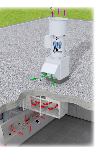
Q<sub>B</sub>= Bypass Flow Q<sub>F</sub>= Fan Flow
