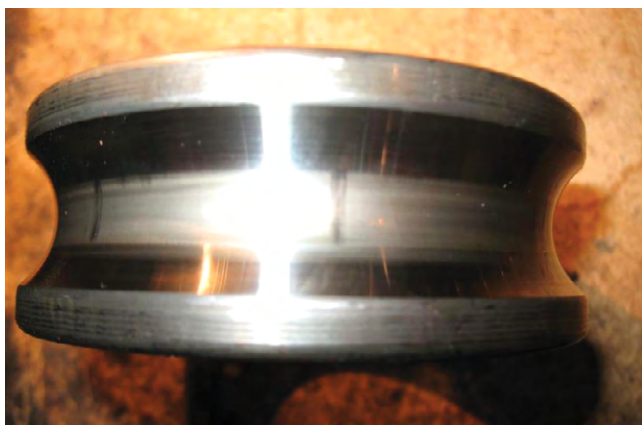
Figure 2. Bearing race exhibiting a "frosted" appearance.
