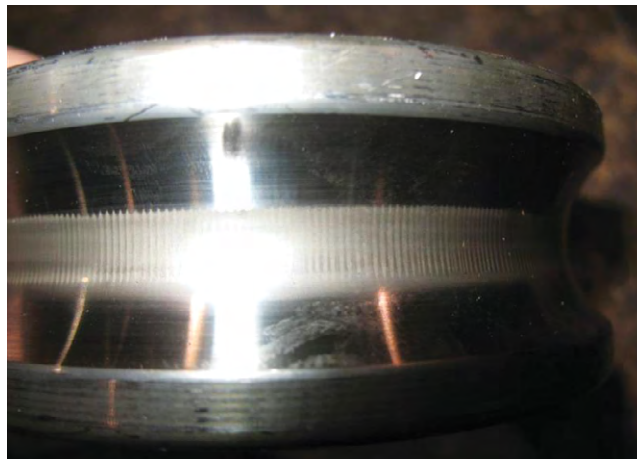
Figure 3. Bearing race exhibiting "fluting".
