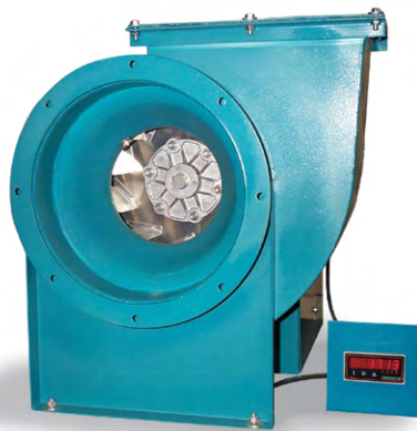
A. Fan operating with unobstructed inlet produces 1713 CFM
