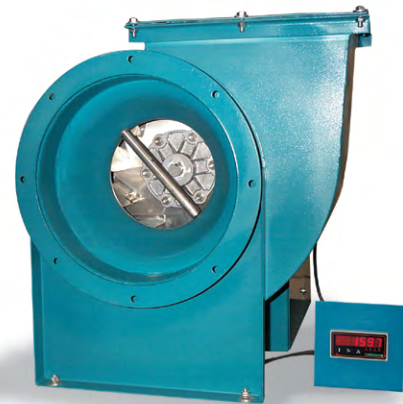
B. Fan operating with obstructed inlet produces 1597 CFM
