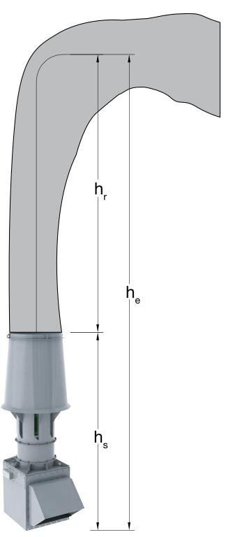
A high Effective Plume Height prevents excessive downwash and prevents the need for unsightly & tall low velocity exhaust stacks.
