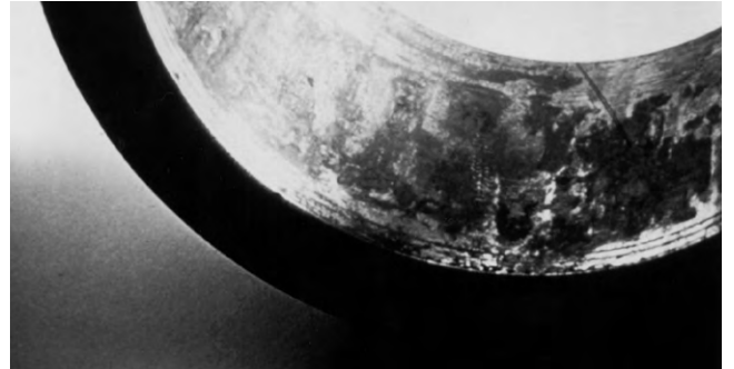
Figure 24. Cracked Inner Race
