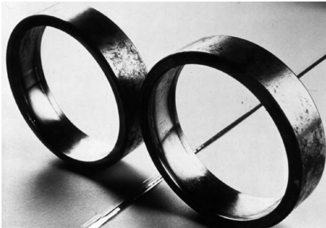
Figure 21. Two Load Zones on the Outer Race
