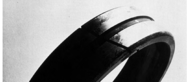
Figure 26. Pits Caused by Electrical Current
