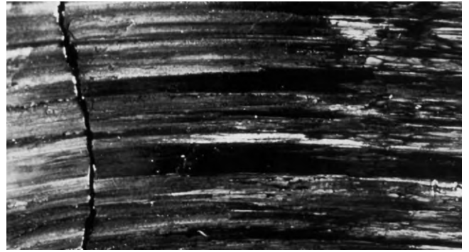
Figure 23. Fretting Corrosion on Bearing Bore
