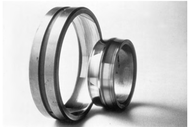
Figure 12. Highly Polished Surfaces Due to Inadequate Lubrication
