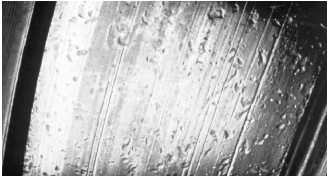
Figure 13. Severe Particle Denting
