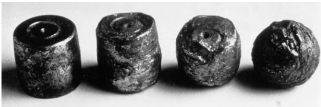
Figure 9. Damaged Spherical Bearing Rollers
