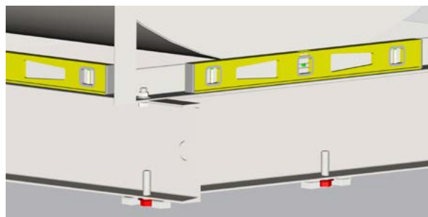
Carefully level the fan on the foundation
