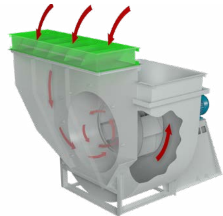
Orientation of Damper Blades Relative to Fan Rotation
