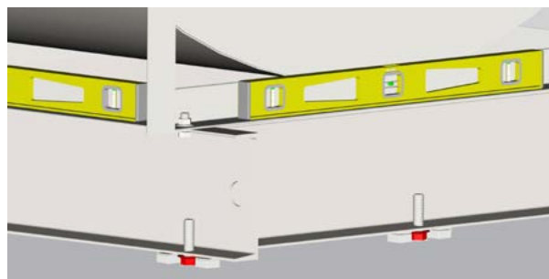
Carefully level the fan on the foundation
