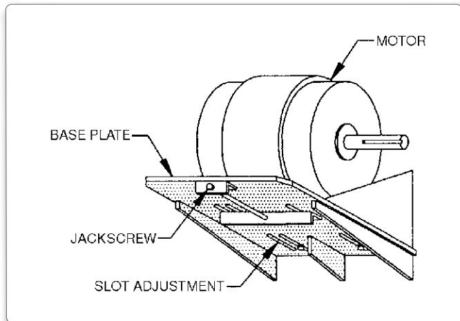
in the illustration above. This arrangement permits adjustment to be made with a minimum of effort, particularly when the motor is of large size.
