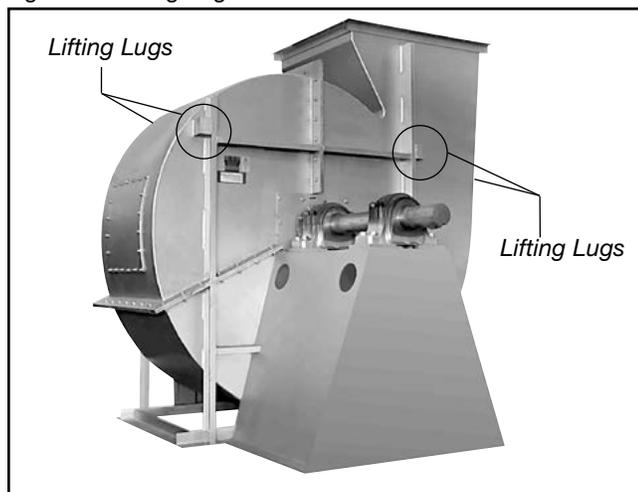
equipment. Units shipped completely assembled may be lifted with slings and spreader bars. (Use well-padded chains, cables or nylon straps.) Never lift a fan by the inlet or discharge flange, shafting or drives, wheel or impeller, motor or motor base, or in any other manner that may bend or distort parts. Never lift with slings or timbers passed through the fan inlets.
