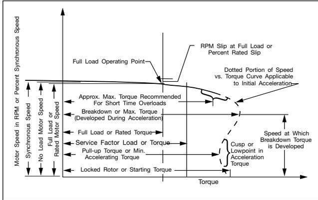
There are many torques that can be obtained from a motor's speed-torque curve:
