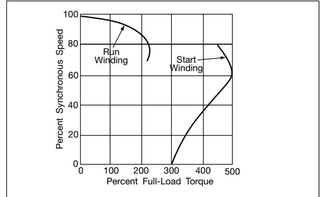
Table 4. Summary Capacitor Start-Capacitor Run Motor Characteristics
