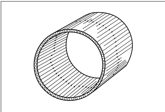
As a rotor turns, the rotor bars cut through the flux lines of the stator magnetic field and voltages and currents are induced in each bar. The magnitude of the voltage and current in a given bar will depend on the magnetic density of the stator field which the rotor bar
