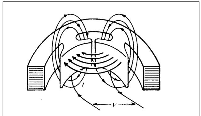
In the completed stator, a magnetic field is created having alternating north and south poles. The number of magnetic poles in the stator, together with the AC line frequency, determines the speed at which the motor will operate.
