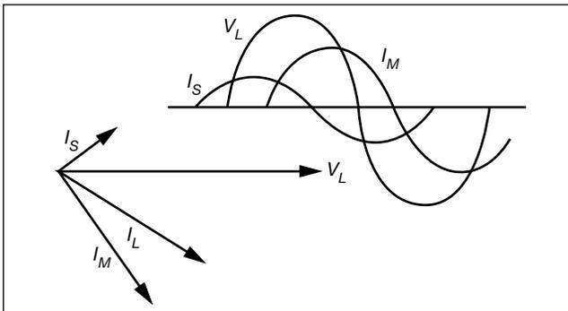
The new result is a time phase shift closer to 90 degrees than with the split-phase motor. A stronger rotating field is therefore created and starting torque is higher than with the split-phase design. Also the vector sum of the main and start winding currents is lower, resulting in a reduction in the inrush current as compared to the split-phase design. Refer to Figure 16.
