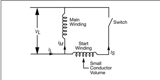
The main (run) winding is designed for operation from 75% synchronous speed and above. The main winding design is such that the current lags behind the line voltage because the coils embedded in the steel stator naturally build up a strong magnetic field which slows the buildup of current in the winding. This relationship between the line voltage and line current is shown in Figure 13.
