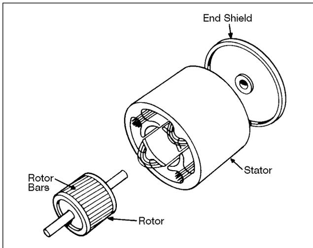
1. **Stator.** The stator is constructed of a set of stacked laminated discs which are surrounded by a stator winding. This winding is connected to the proper power supply (voltage, phase and frequency) and produces a magnetic field that revolves around the motor at a speed designated "synchronous."
